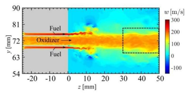
Flow velocity in the fuel/oxidizer injectors and combustion chamber during combustion oscillations in a model of a rocket engine. (Courtesy: Hiroshi Gotoda)
